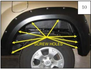
Position flare on fender and install eight supplied hex head screws (SW1-0036) through holes in flare and into factory holes.
